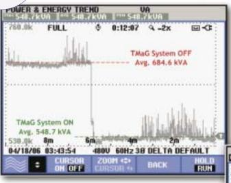
Below are actual meter display results of a PureMon1cs™ TMαG System™ that shows dramatically improved distribution system efficiency and reduced power demand on a 1000kVA main distribution transformer.
